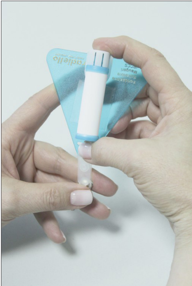
Fit the diffusive body to the adapter by pushing it till you hear a clicking sound.
