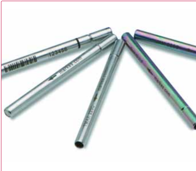
Sorbent tubes are a convenient way of sampling vapours for analysis by TD-GC-MS.
